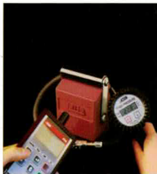
6. Trigger Sensor with ATEQ TPMS tool
