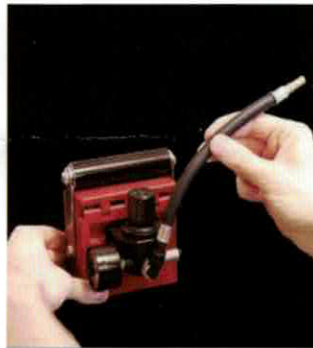
4. Connect Shop air to the push on fitting
