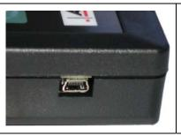
The **USB** connection allows firmware updates to be installed onto the tool using the **WebVT** software (only in boot mode, see below). TPM Sensor results can also be printed using this software.
