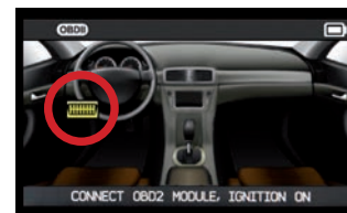
Pictures indicate the OBDII location in the car.
