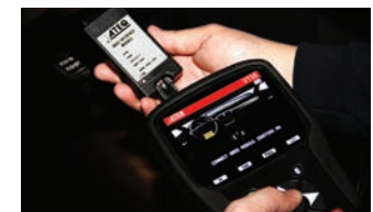
The tool reads TPMS DTC codes on applicable vehicles.
