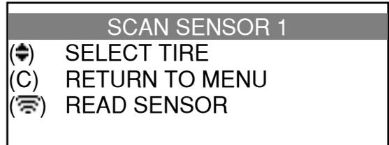
Here you are ready to read the first wheel as shown by the words "Scan Sensor 1". To change wheels, use the "up" and "down" arrows.
