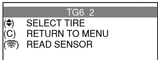
To read the second sensor, simply press "OK". The screen then shows that VT TRUCK is ready to read the second sensor: "TG6 2".
