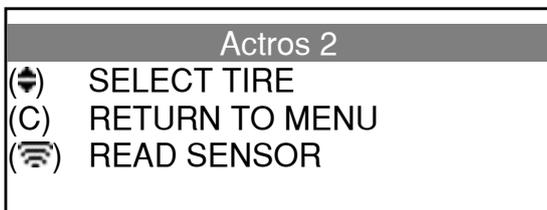
To read the second sensor, simply press "OK". The screen then shows that VT TRUCK is ready to read the second sensor: "Actros 2".
