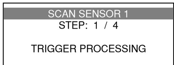
VT TRUCK successively transmits the different TPMS sensor wake-up frames. The step in progress is shown as "Step x / 4".
