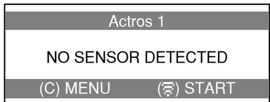
The TPMS sensor does not work, no sensor is present on the tyre being tested, or VT TRUCK is incorrectly positioned or too far from the sensor.
