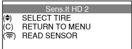
To read the next sensor, simply press "OK". The screen then shows that VT TRUCK is ready to read the second sensor: "Sens.It HD 2".
