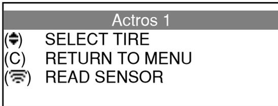
Press "Sensor Activation" (green) to launch the process of reading the TPMS sensor.
