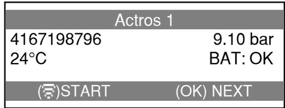
The sensor was read successfully. The screen displays: the ID of the sensor, the temperature inside the tyre, the pressure measured and the status of the TPMS sensor battery.
