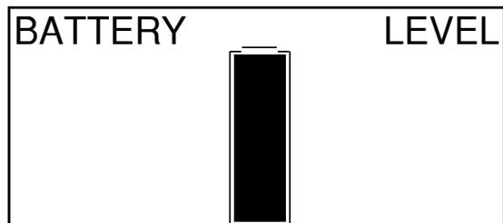
When the battery is charged, the status bar is full and the "**CHARGE**" indicator lights up in green.
