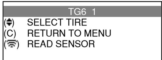
Press "Sensor Activation" (green) to launch the process of reading the TPMS sensor.
