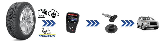
The embedded RFID tag delivers a unique tire ID number from which additional tire data can be retrieved in the cloud. Tire data are then copied to the ATEQ tool and transferred to the TMS or TPMS sensor. When mounted on a vehicle, the TPMS or TMS sensor will continuously transmit all its contained data to the vehicle ECU.
