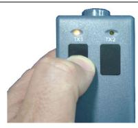
2 - Start the cycle by pressing and releasing the left key (TX1)
