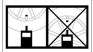
1 - Put the VT15 in front of the tire near the sensor
