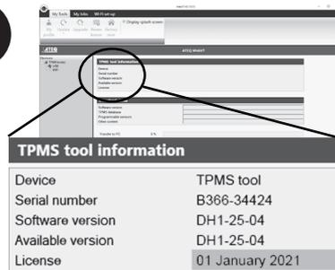
Connect your tool to your PC via USB cable. Once connected, all of the tool's information will be displayed, including the software subscription date.
