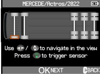
The data of the first sensor in the sensor set to be copied is read out
