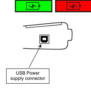
When the battery is low, the "status bar" appears every 10 seconds. This display will stop when the battery loses power.
