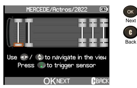
The truck configuration you made with the configurator, refer to page 13, is displayed. You are ready to check sensors.
