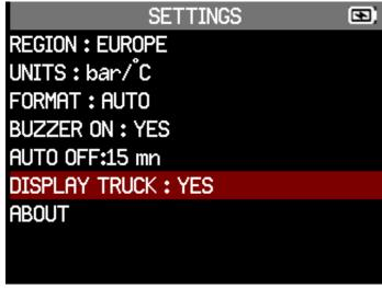
Displays or clears the truck in the **Check Sensor** and **Program Sensor** sections
