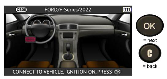
The tool will read the vehicle's reference TPMS data from the ECU.
