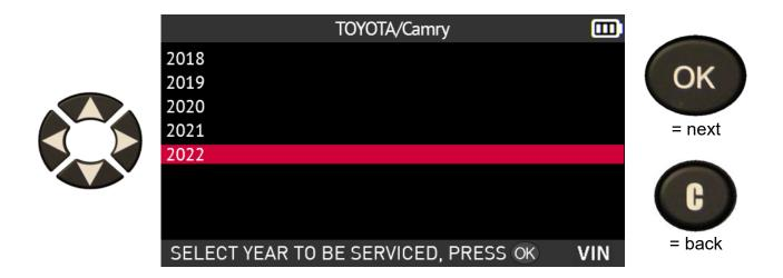
If the year in which the vehicle was put into service is unknown, select the **VIN** icon in the lower right-hand corner of the screen using the arrow buttons. Press **OK** to confirm your choice.
