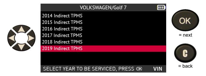
The tool then indicates the relearn procedure to be followed. Use the up and down arrow keys to scroll through the screen and read the complete procedure.
