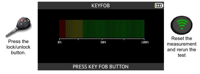
The tool will wait for a signal and then display the strength of the signal it receives.
