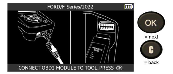
Connect the OBD-II module to the vehicle's OBD port.
